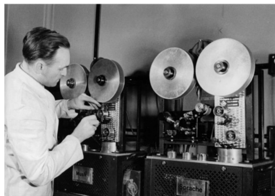
Figure 2.1 German magnetic tape recorders photographed in 1941. Bundesarchiv, Bild 183–2007-1026–500 / CC-BY-SA
